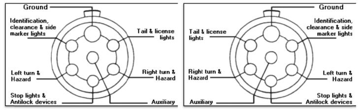
Warning: It is necessary to use electrical tester to establish proper match of vehicle's wiring to trailer's wiring. Failure to do so may cause damage.
